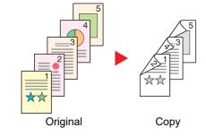
Produces two-sided copies from one-sided originals. In case of an odd number of originals, the back side of the last copy will be blank. The optional duplex unit is required.
