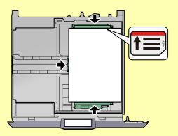
2 Insert the appropriate paper size card in the slot to indicate the size of the paper inside.
