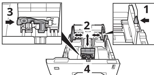
+ If the paper is loaded without adjusting the paper length guide and the paper width guides, skewed paper feeding, and a paper jam will occur.
