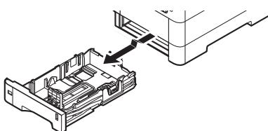
**2** Adjust the paper length and width guide to the paper size required.
