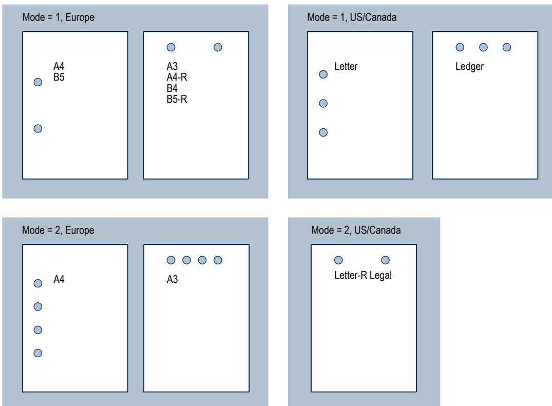
The *mode* parameters of 51, 52, 61, 62, 71, and 72 are valid for some copier models only. These parameters allow to position the holes in either of the left, right, and top sides of the page by logically aligning the page in reference to the punched holes.
