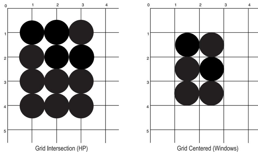
Assuming a rectangle extending from coordinate (1, 1) to coordinate (3, 4), a different result is obtained depending on each pixel placement mode. Grid intersection is default to HP PCL; and grid centered mode is used by Microsoft Windows.
