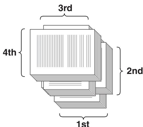
The RCLT command is available when printing using A4, B5 and letter size paper. During printing, the same size paper must be loaded into two separate cassettes. For example, Portrait (A4) and Landscape (A4-R) would be used when printing onto A4 paper. The MP tray can also be used as a paper source.
