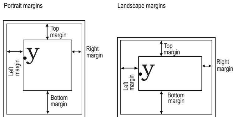
If the printing system cannot adjust the margins as described above, it sets them to the edge limits. For example, if you set a top portrait margin greater than the paper width, then switch to landscape orientation, the printing system resets the top margin to zero.
