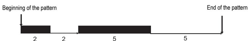
The maximum number of pairs of dash and space allowed for a SDP command is 10. If the dash pattern begins with a space, 0 must be specified for the first *dash* value (*dash1*). To end the pattern with a dash, the last *space* value may be omitted.
