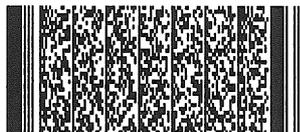
The bar height is twice as high as the element width. Since the default bar height is a triple of the element width, the barcode aspect ratio is now in ratio of 2:3. (See XBCP 6.)
