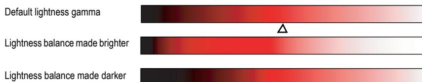
Varying the lightness gamma allows the lightness of the image to vary. (You can achieve lightness variation, such as making dark images brighter by reducing low lightness areas, for example.)
