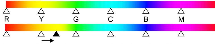
If this command is issued to rotate a particular hue when all hues are rotated, the hues are controlled after they are reset to their default state. The HUE command is enabled for all color spaces, all color modes and all monitor simulation modes. If ink simulation is set to other than NONE, the HUE is disabled.
