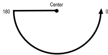
Negative values are acceptable for angle. For example, an angle of 315 degrees is the same as -45 degrees.
