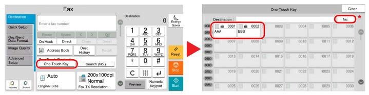
The [No.] key has the same function as [Search (No.)] displayed on the touch panel. Use to directly enter a number with the numeric keys, such as specifying a transmission address using a one-touch key number, or calling up a stored program using the program number. For information on one-touch key numbers, refer to the following:
