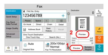
The machine starts scanning the original. When scanning is completed, the preview image appears on the panel.
