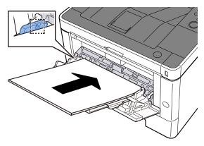
Insert the paper along the paper width guides into the tray until it stops.
