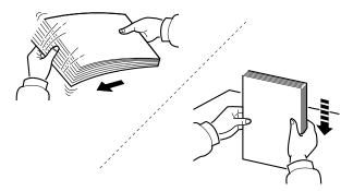
Fan the paper, then tap it on a level surface. In addition, note the following points.
