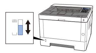
Remove the paper from the cassette once if there is no improvement, turn it over and reload it, or change the loading direction by rotating the paper 180 degrees.
