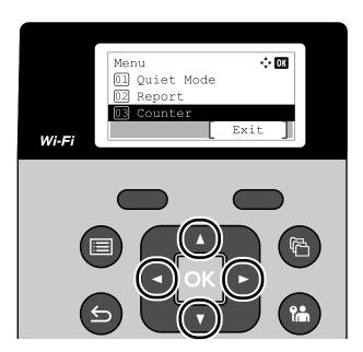
When [OK] is displayed, selecting the [OK] key will confirm the selection. Selecting the [Back] key will return to the previous level in the menu.
