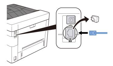
2 Connect the other end of the cable to the hub.
