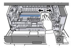
7 Slide the upper charger cleaner knob of the Drum unit to the left and right two or three times.
