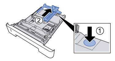
2 Adjust the position of the paper width guides located on the left and right sides of the cassette. Press the paper width adjusting tab and slide the guides to the paper size required.
