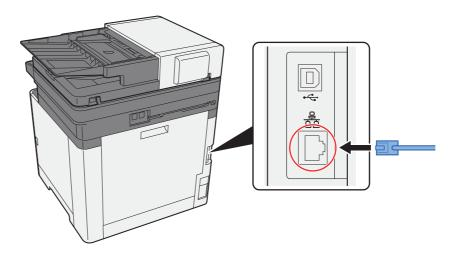
2 Connect the other end of the cable to the hub or the PC.
