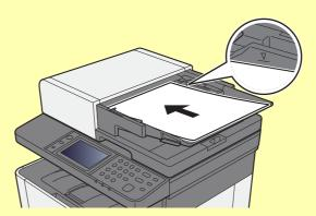
Ensure that loaded originals do not exceed the level indicator. Exceeding the maximum level may cause the originals to jam.
