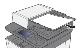
Open the front cover and remove any jammed paper.
