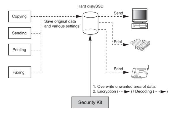
If the security kit is introduced while the hard disk and SSD are installed in the machine, the destination where data received by FAX is to be saved is changed from SSD to hard disk. If you want to change the destination to SSD, contact your dealer or service technician.
