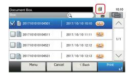
When the security kit has been installed and is running properly, Icon (1) appears in the touch panel while unneeded data is being overwritten.
