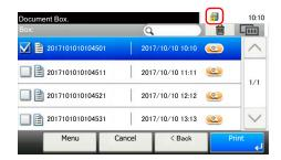
When the security functions has been installed and is running properly, Icon ( ) appears in the touch panel while unneeded data is being overwritten.
