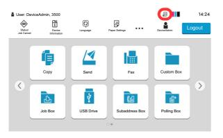
In Security Mode, the security functions have been properly installed and is running. The hard disk icon appears on the top right side of the touch panel in Security Mode.
